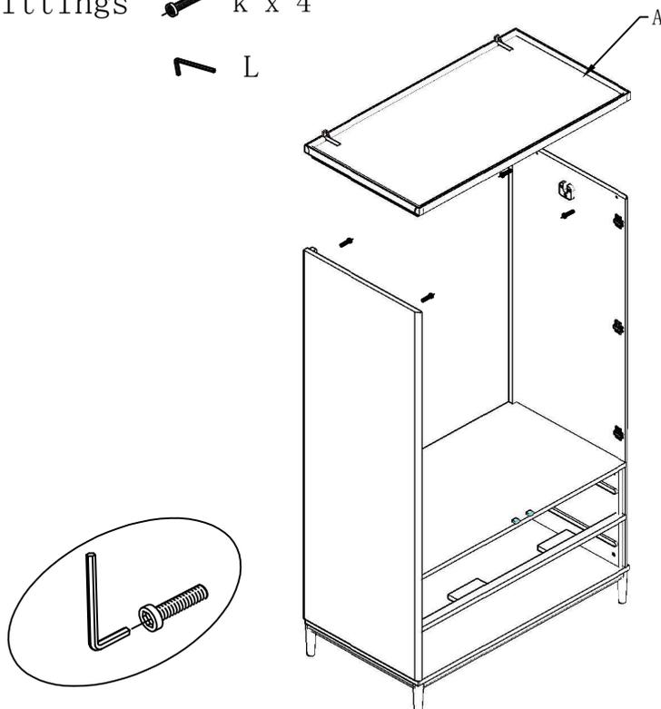
3. First insert the back panel J1 and J2 into the back panel rail I, Then attach the back panel J1 and J2 onto the back side of wardrobe unit by using 20pcs 20mm screws M and attach the back panel rial I onto the unit by using 2pcs 25mm screws N as shown below.
