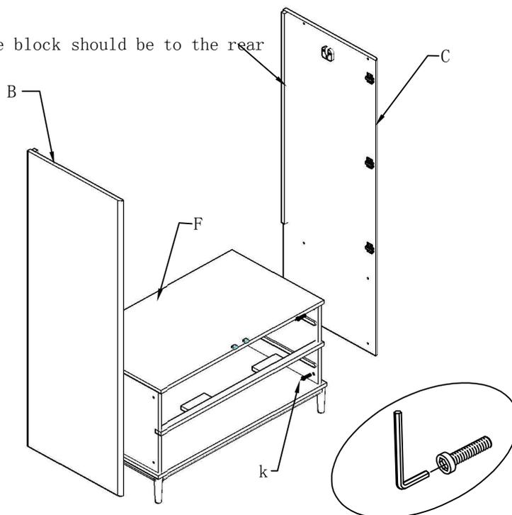
2. Attach the top panel A onto the left side panel B and right side panel C by using 8 pieces 25mm bolt K with the allen key L as shown below.
